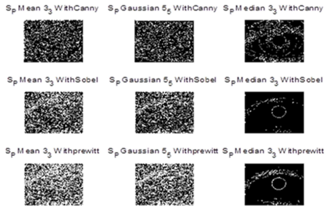
Figure 6. Applying mean, median and Gaussian filter to remove salt and pepper noise.
