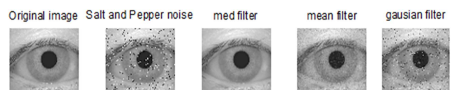
Figure 8. Removal of salt and pepper noise of image using median, mean and Gaussian filter.
