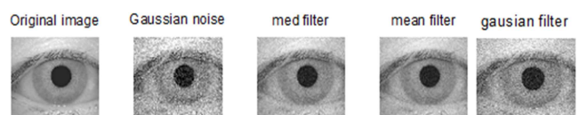
Figure 9. Removal of Gaussian noise of image using median, mean and Gaussian filter.
