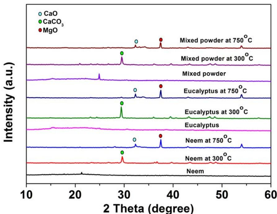
Figure 5. XRD spectra of the various samples.
