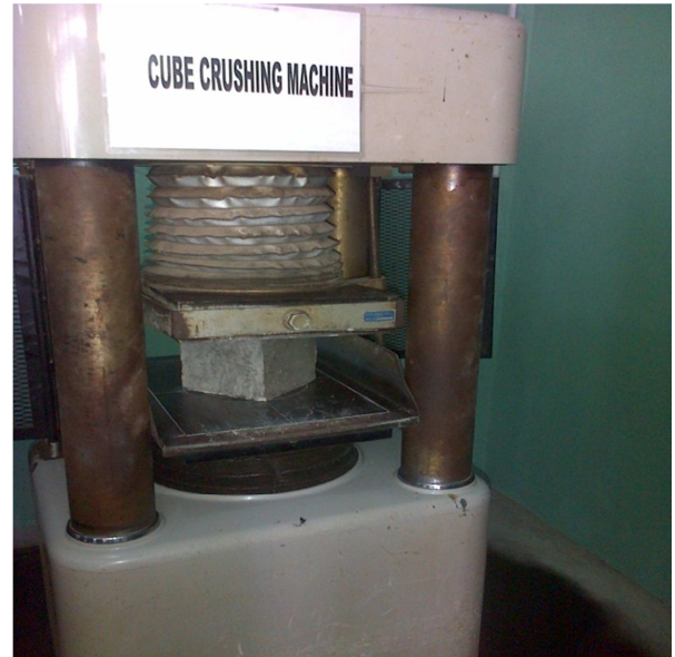
Plate 2. The Concrete cube under crushing
