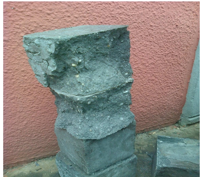
Plate 3. Samples of the crushed concrete cubes
