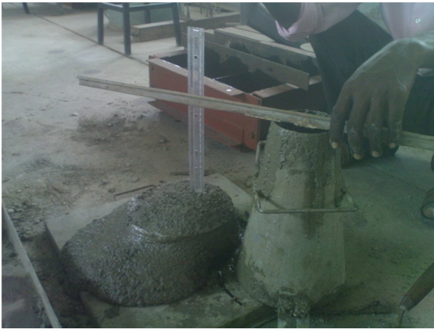
Plate 1. Determination of Slump Workability
