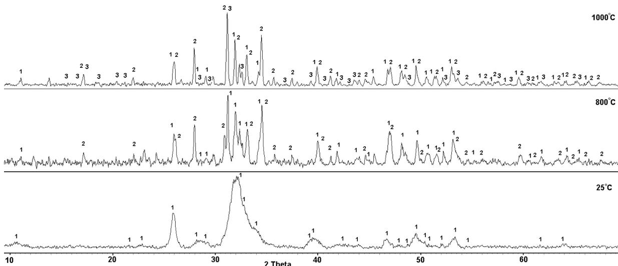
*Fig. 2. The X-ray diffraction patterns of HAP produced at ISSC UB RAS at different annealing temperatures: 1 -  $\text{Ca}_{10}(\text{PO}_4)_6(\text{OH})_2$ ; 2 -  $\beta\text{-Ca}_3(\text{PO}_4)_2$ ; 3 -  $\alpha\text{-Ca}_3(\text{PO}_4)_2$ .*
