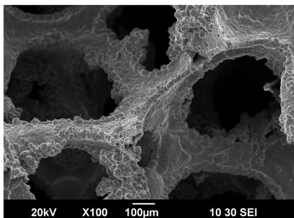
Fig. 3. The micrograph of highly porous honeycomb nickel.
