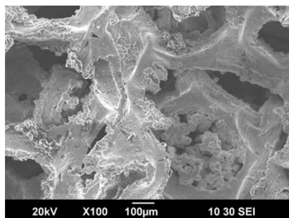
Fig. 4. The micrograph of the surface of highly porous honeycomb nickel upon application of titanium coating.
