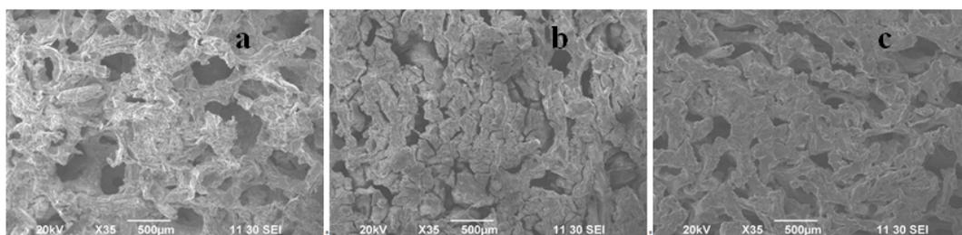
**Fig. 6.** The micrographs of the biocomposite prepared by different methods: method 1 (a), method 2 (b), method 3 (c).
