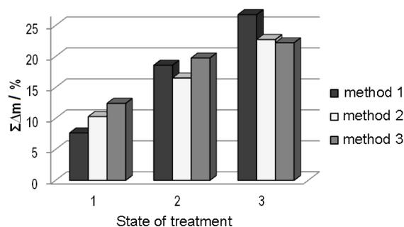
Fig. 5. The variation in the biocomposite mass as a result of dosed stepwise saturation of highly porous titanium nickelide with HAP with the use of different methods.
